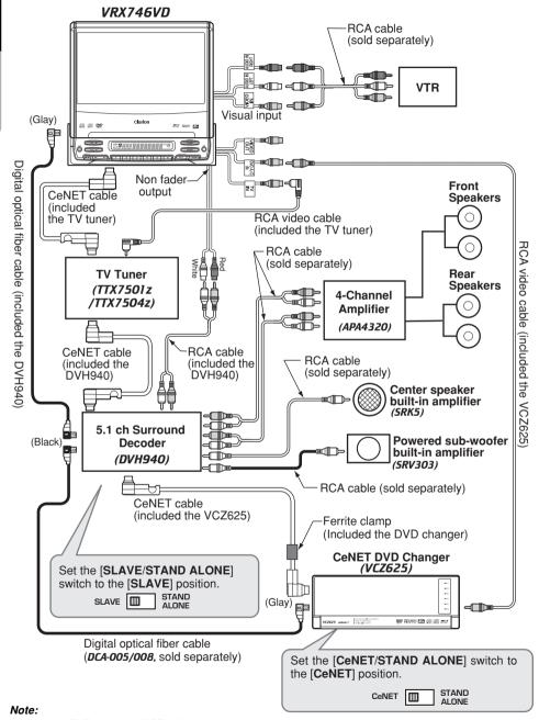
When the DVD changer (VCZ625) is connected via optical cable, no sound will be output if AUDIO OUT is switched to ANALOG on the changer's "GENERAL SETUP" menu.
